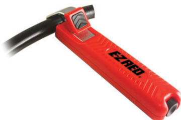
Adjustable Battery Cable Stripper with adjustable blade, strips insulation jacket from cable, range of 8 gauge to 4/0 AWG EZ-793CS
