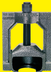
H.D. Universal Joint Puller used with 1" dr. impact gun. Fits virtually all class 7 & 8 H.D. truck & machinery drive lines, without damaging bearing cups, yokes, joints, etc. TGT-10102
