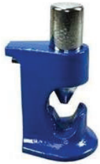
Hammer Indent Type Battery Cable Crimping Tool • Spring loaded pin • Cast steel body, • 8 Gauge to 4/0 AWG EZ-B790C
